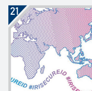
Relief with Line Width Modulation (2 in 1 security features)
